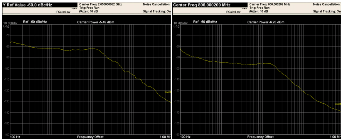
Figure 29 Measured phase noise a) at LTE band 7 and b) LTE band 20
